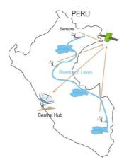
Figure 1. Mission concept. Data from polluted water is sent to a Central Hub in Lima through satellites.
