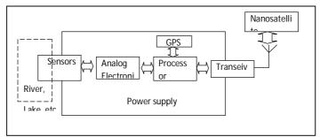
Figure 3. Autonomus multi-sensor system (AMSS) diagram.
